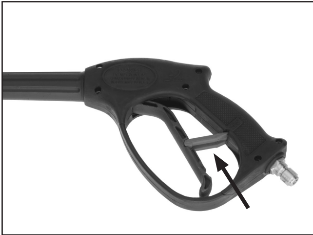
Figure 10. The spray gun in the locked position.
